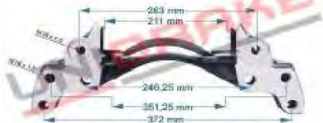
6828 / Caliper Carrier / DAF LF55 - LEFT WABCO CARRIER
