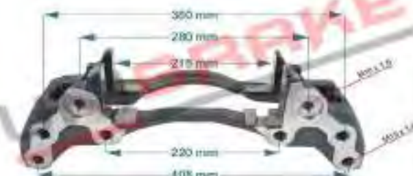
6806 / Caliper Carrier / MAN TGX-TGS / RIGHT WABCO CARRIER
