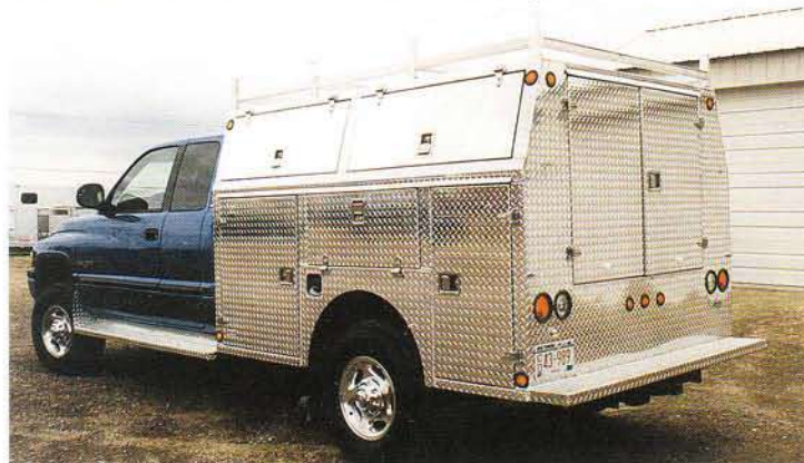
21. All types of customizing available including: shelving, transverse compartments, roll out trays, double pan doors, door stops, special latches, hanging hardware, and interior lighting. Our rescue bodies have been used and approved by the U.S. Army.
