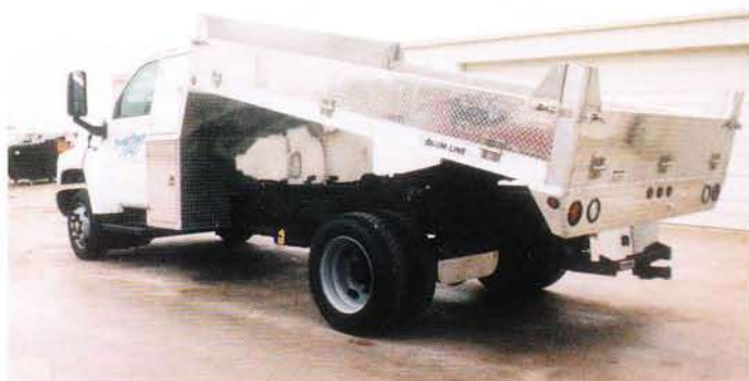
16. ALUM-LINE dump body platforms are heavy duty. Special strength options include; 1/2" thick outside framing with 1 1/4" extruded flooring. Channel long sills and heavy duty bulkheads complete the package.
