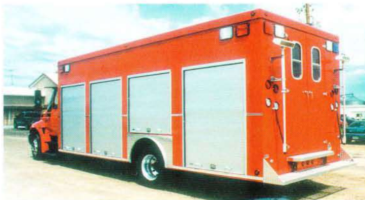
20. Rescue body with 60" box height. Four compartments per-side and finished in .125 smooth aluminum painted sides. Rear step bumper and rolled fender flares. More information is available on our complete line.
