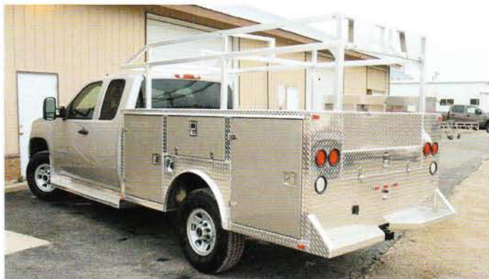
19. One of our most popular set ups. Compartment height at 40" with overhead ladder rack and step bumper. Other popular options include 4" deep flip top compartments on top, adjustable shelving, slide out trays, painted doors and much more. All models available in smooth or treadbrite aluminum construction.
