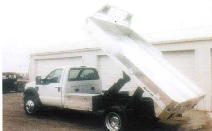
17. Bed capacities up-to 12 ton are available. Our extruded flooring offers easy dumping. Permanent solid sides come in a variety of heights and in either smooth, extruded, or diamond plate material.
