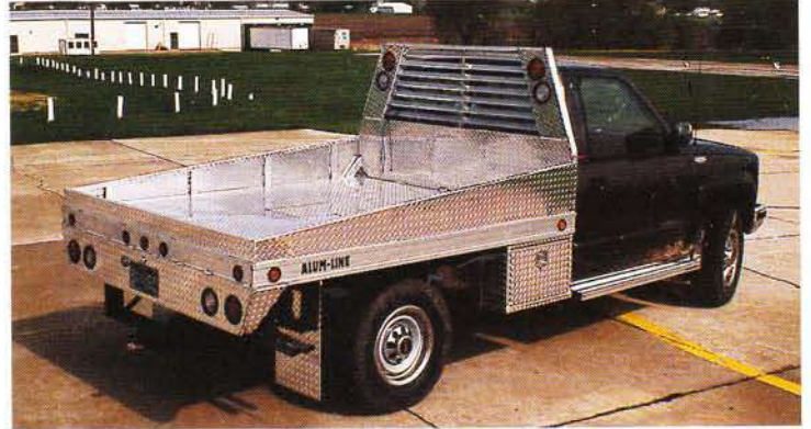
7. Our most popular truck bed package. Louvers and lights, tapered side boards, underbody tool boxes, mudflaps, and fifth wheel trap door.
