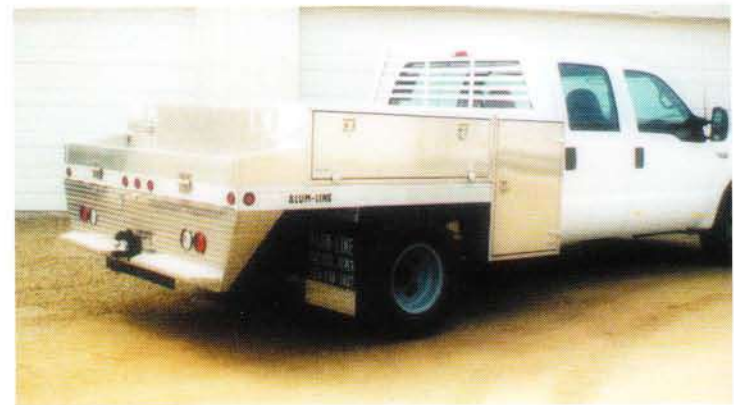
2. Equipped with optional above bed tool boxes, upright front tool boxes, rear step bumper, louvered bulkhead and short sides. You can build a body your way.
