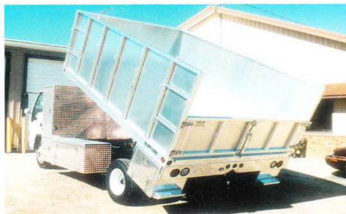
18. Special dump body set up using a "Back Pack" behind the cab. "Back Packs" provide extra storage for large tools, shovels, etc.. Please note the removable stake sides for multiple use.
