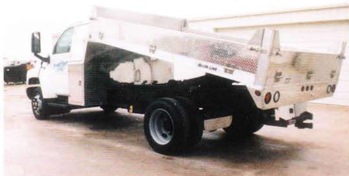
16. ALUM-LINE dump body platforms are heavy duty. Special strength options include; 1/2" thick outside framing with 1 1/4" extruded flooring. Channel long sills and heavy duty bulkheads complete the package.
