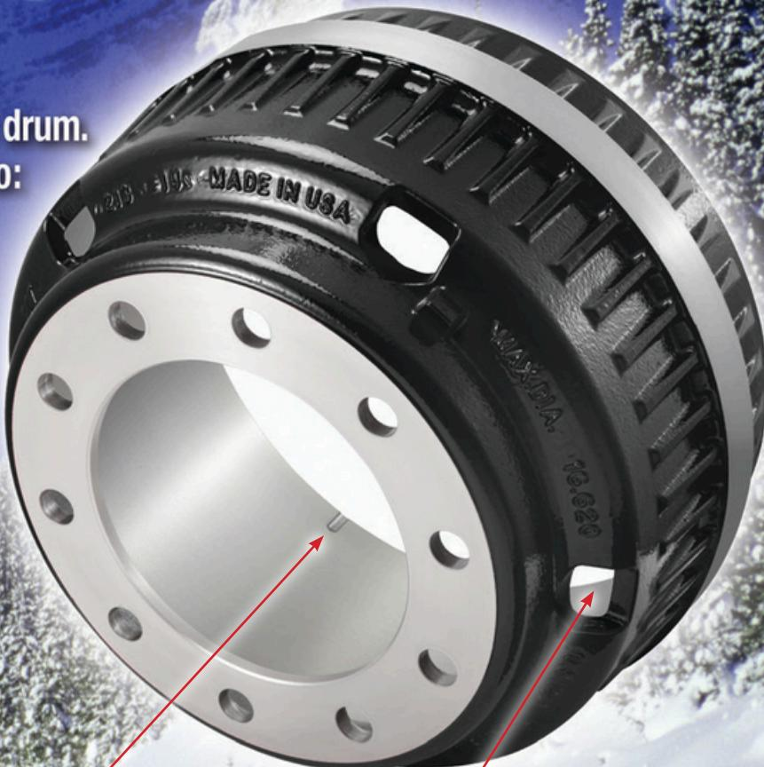
NEW patented wear indicator saves time and helps you get maximum life from your drum to cut maintenance time and cost.
