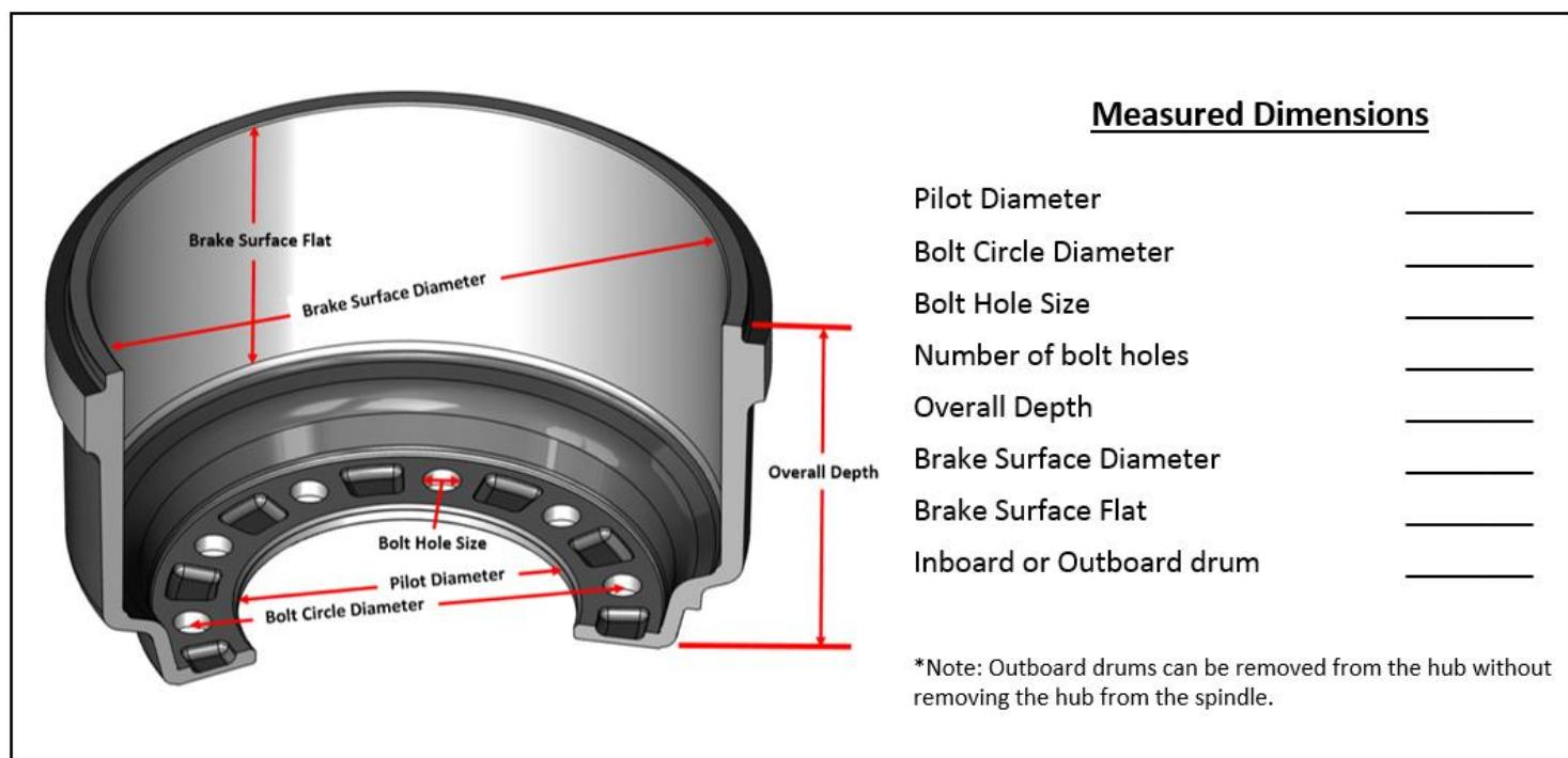
\*Verify the weight of the replacement brake drum is comparable to the weight of the brake drum being removed from the vehicle. If you have any questions, please visit Webb's Training Toolbox at [http://www.webbwheel.com/aftermarket/training\\_toolbox.html](http://www.webbwheel.com/aftermarket/training_toolbox.html) for additional information.
