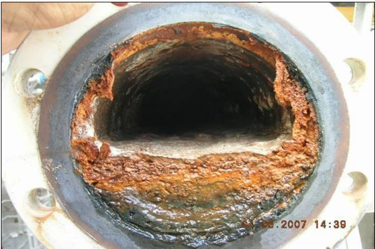
Above: Sewer pipe gravity flow main with narrowing from fats, oils and greases.
