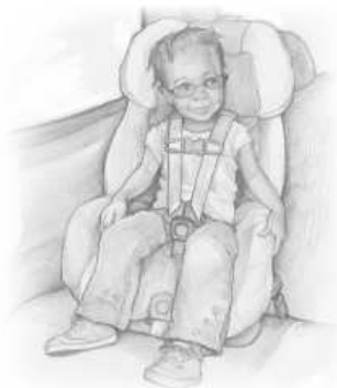
FIGURE 4. Forward-facing car safety seat with harness.
