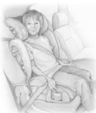
FIGURE 5. Belt-positioning booster seat.
