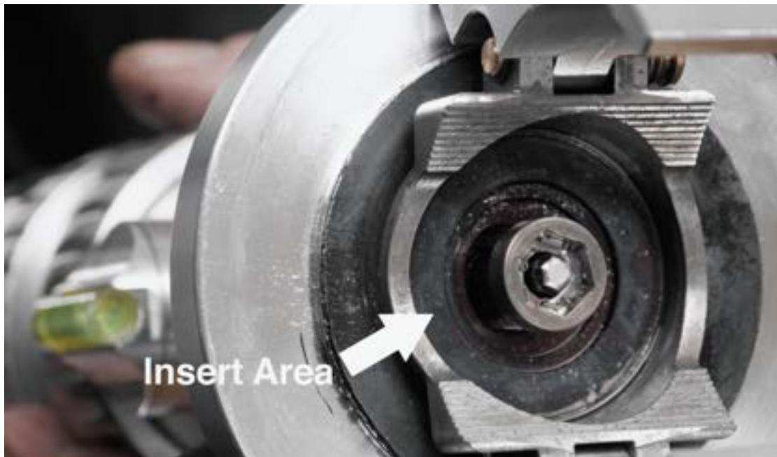
Snapdrill and the battery drill need to be connected in order to insert hole saws.
