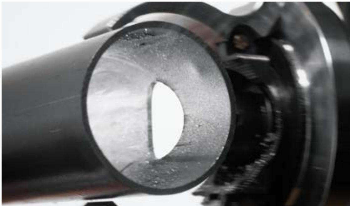
Once drilling is completed, do not yet return the hole saw, loosen the handles. First with two hands, then with one hand while holding the battery drill with the other. Remove Snapdrill from the pipe.
