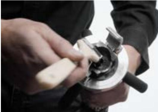
Regularly clean Snapdrill for metal shavings. Use a brush or a magnet. Do not use pressured air.
