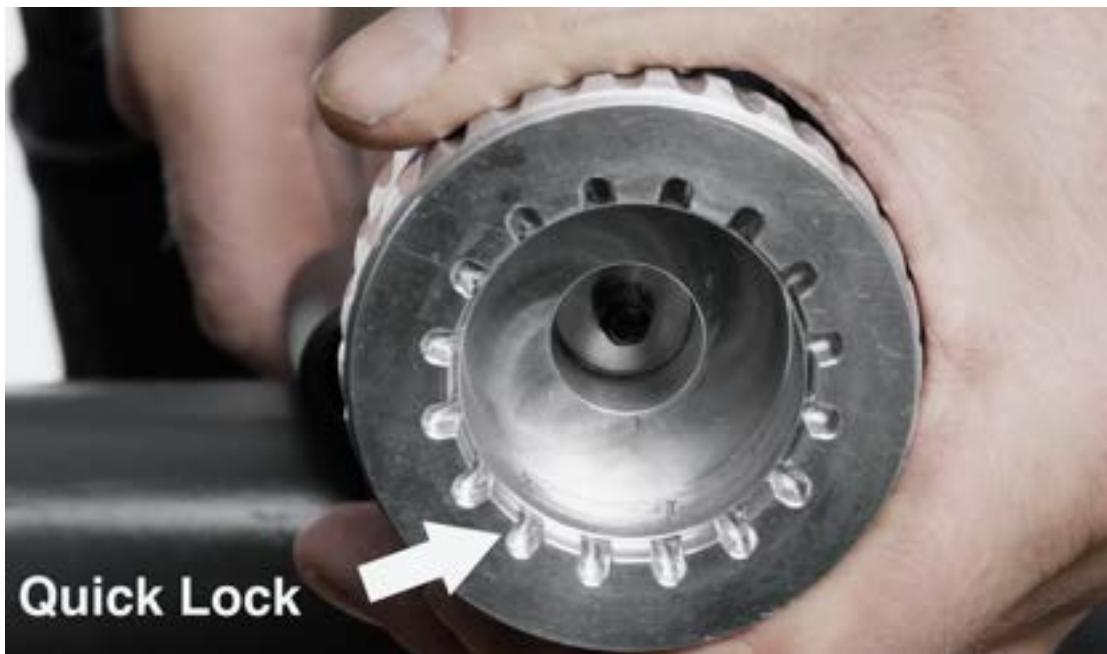
Snapdrill connects directly to its drive unit with the quick lock.
