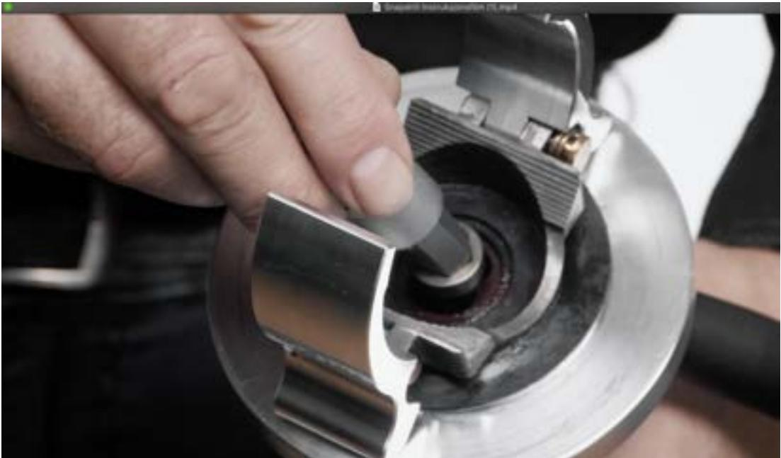
Remove the bolt. Use the included socket and flex handle.
