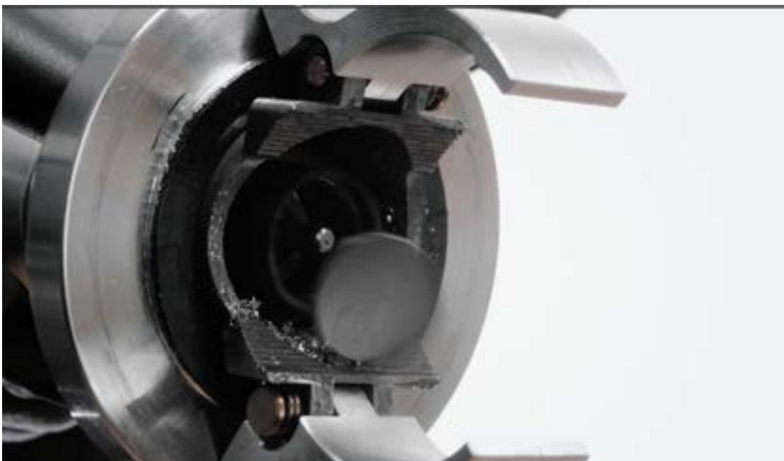
Tighten the feed nut for and return the hole saw for removal of debris.
