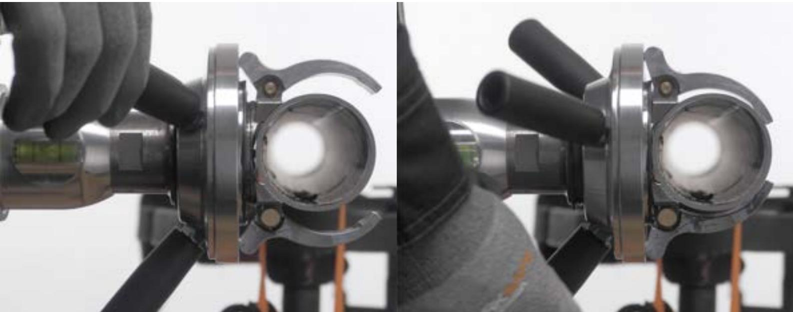
Extend the foldable handles, open the clamp, and tighten Snapdrill to the pipe.
