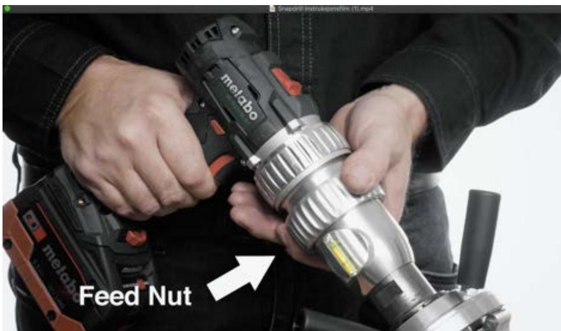
Tighten the feed nut. Pull the trigger and let the insert area come forward.
