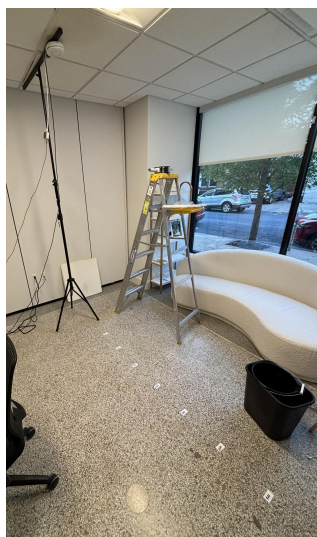
One of the testing setups in a commercial setting, tape was put on the floor to make it easy to record distance from the sensor.
