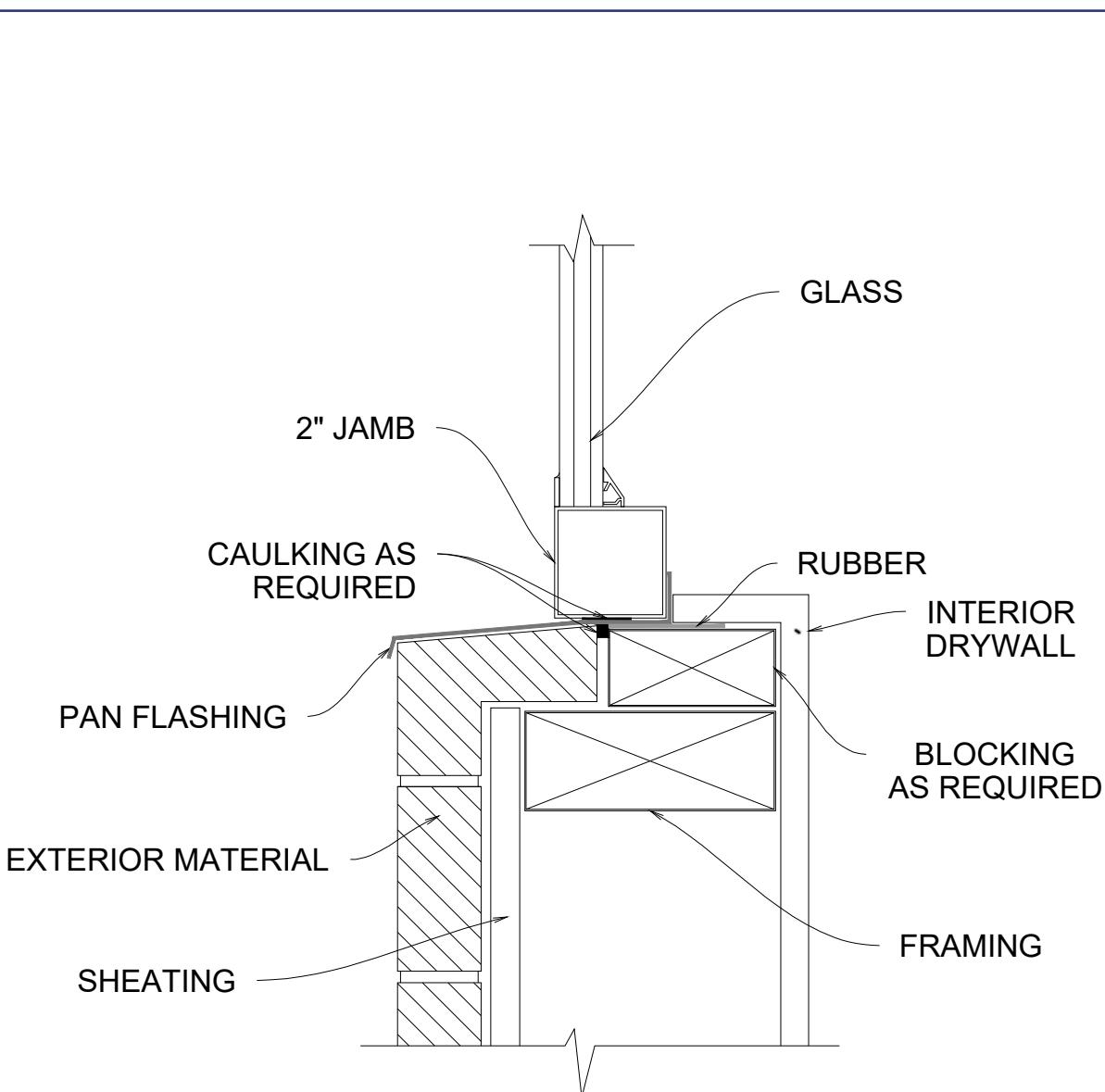
These details are recommendations only and for design consideration only. They should not be used for construction and a design professional should be consulted for final construction drawings. All units should be waterproofed both after the building wrap, and on completion of the exterior material.
