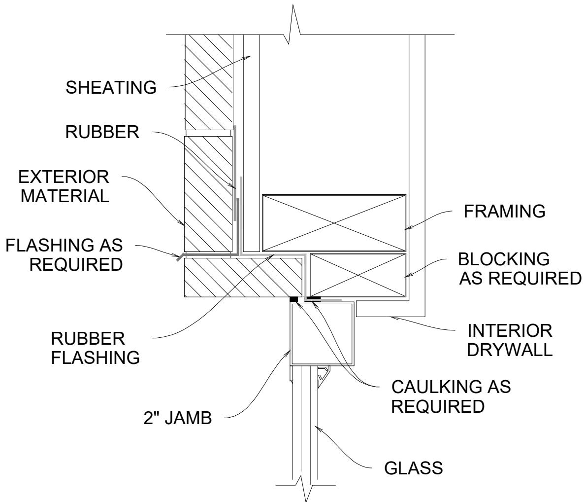
These details are recommendations only and for design consideration only. They should not be used for construction and a design professional should be consulted for final construction drawings. All units should be waterproofed both after the building wrap, and on completion of the exterior material.
