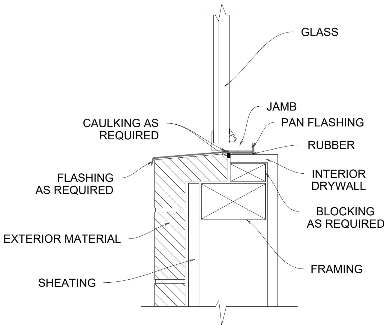
These details are recommendations only and for design consideration only. They should not be used for construction and a design professional should be consulted for final construction drawings. All units should be waterproofed both after the building wrap, and on completion of the exterior material.
