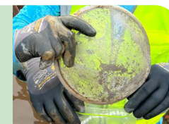
Fig 5: Transferring drill cutting samples into a resealable bag
