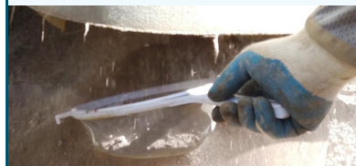
Fig 2: Demonstration of drill cutting sample collection in air drilling
