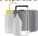
Fig 5: Sand Content test kit
