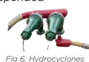
Fig 6: Hydrocyclones for removing sand from drilling fluid
