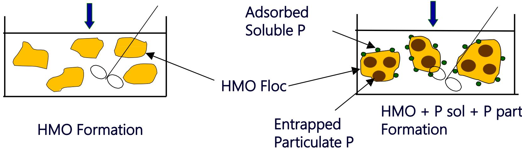
Therefore, good mixing is required for HMO(Floc) formation and chemical dose optimization
