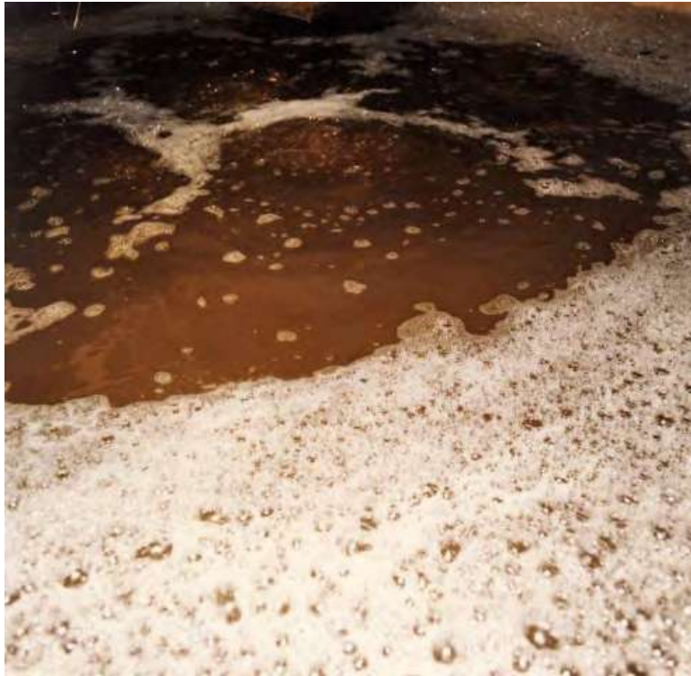
Fig. 11 Barley immersed in steep in Village Maltings, photograph by Kevin Dwyer, 1994.
