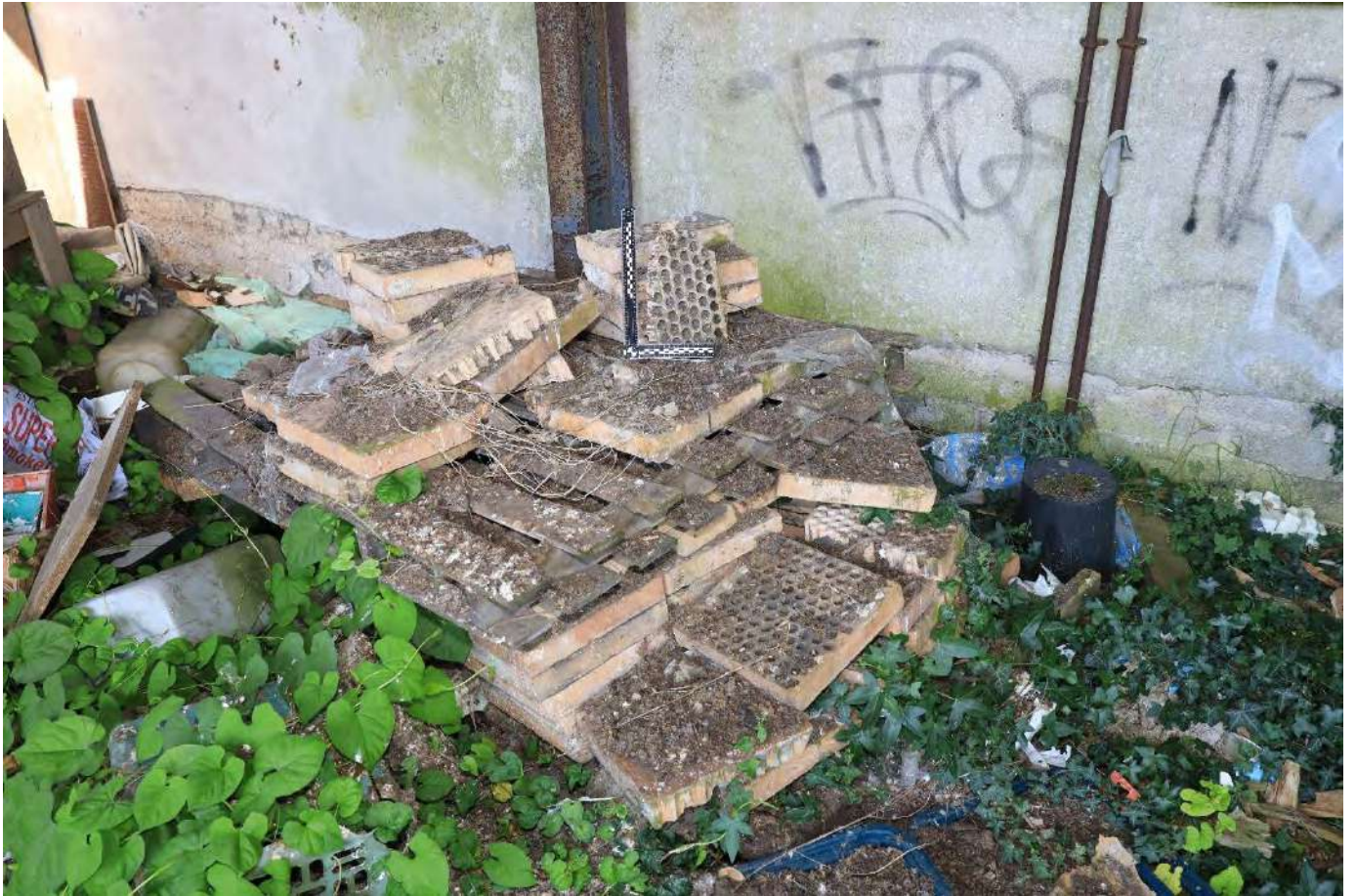
Fig. 43 Perforated ceramic ('Worcester') kiln tiles, stored in former drying shed of the 1960s silo.
