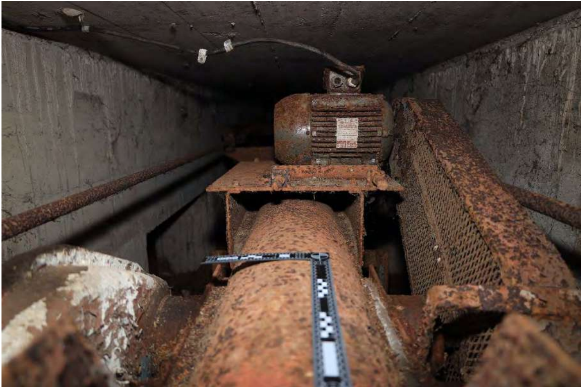
Fig. 87 Interior of opening in south wall of grain silo for hopper regulator, showing unit driven electric motor, with chain drive (in metal casing) on the right.
