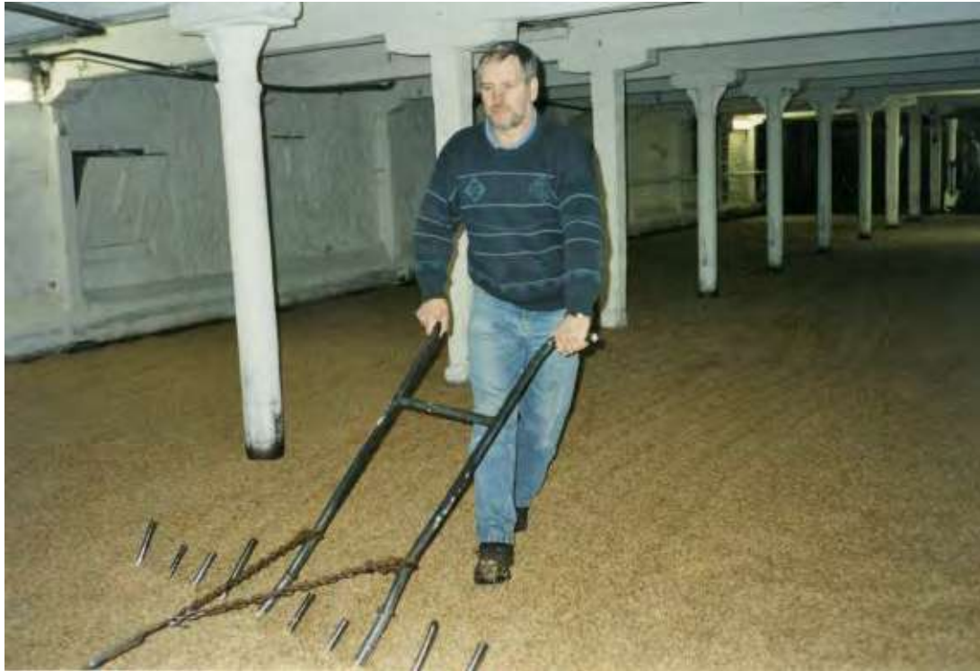
Fig. 15 William Ahern, using a ‘plough’ in the 1900 extension to the Village Maltings, in April 2001. Photo: Ursula O’Mahony.
