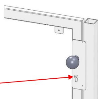
In the case of the automatic door, you must first decouple the motor from the door drive. To do this, push the flap on the front side of the motor upwards and turn the pin according to the picture on the motor. Then unlock the lock with the triangular key (plastic) and open the door manually. Open the door only when the door drive is decoupled, as otherwise the gearbox will be damaged!
