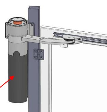
Motor unlocking device
