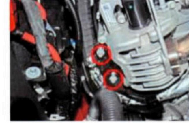
Step 11: Remove the two clips on the heat shield that are located on the passenger side under the egr cooler.
