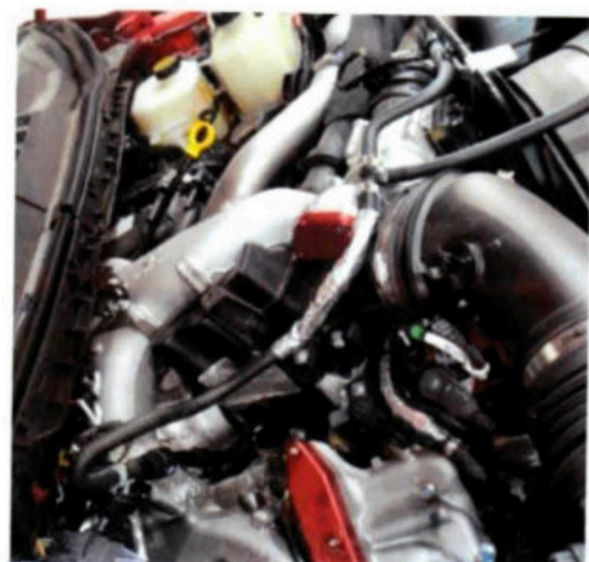
Step 20: Reconnect the PCM harness. Make sure the plugs are fully seated.
