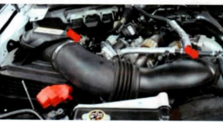
Step 4: Remove the left most hose from the coolant Tee. The coolant hose from the top of the quick connect coolant line at the metal stand pipe will reconnect here.
