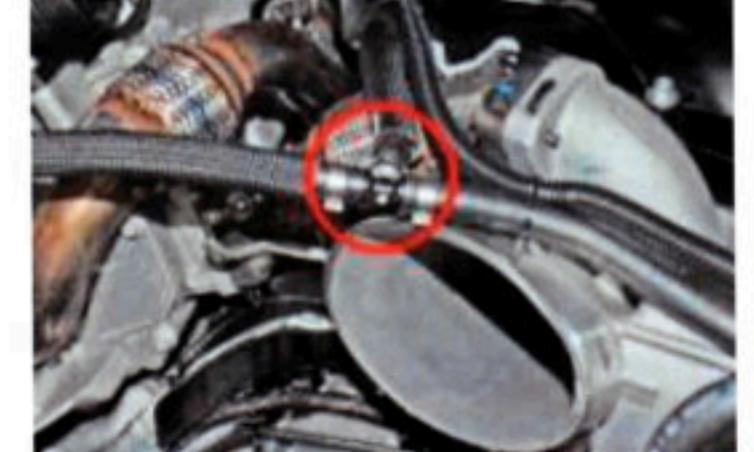
Step 5: Disconnect the quick connect coolant line from the metal stand pipe that is between the egr cooler and the intake manifold.
