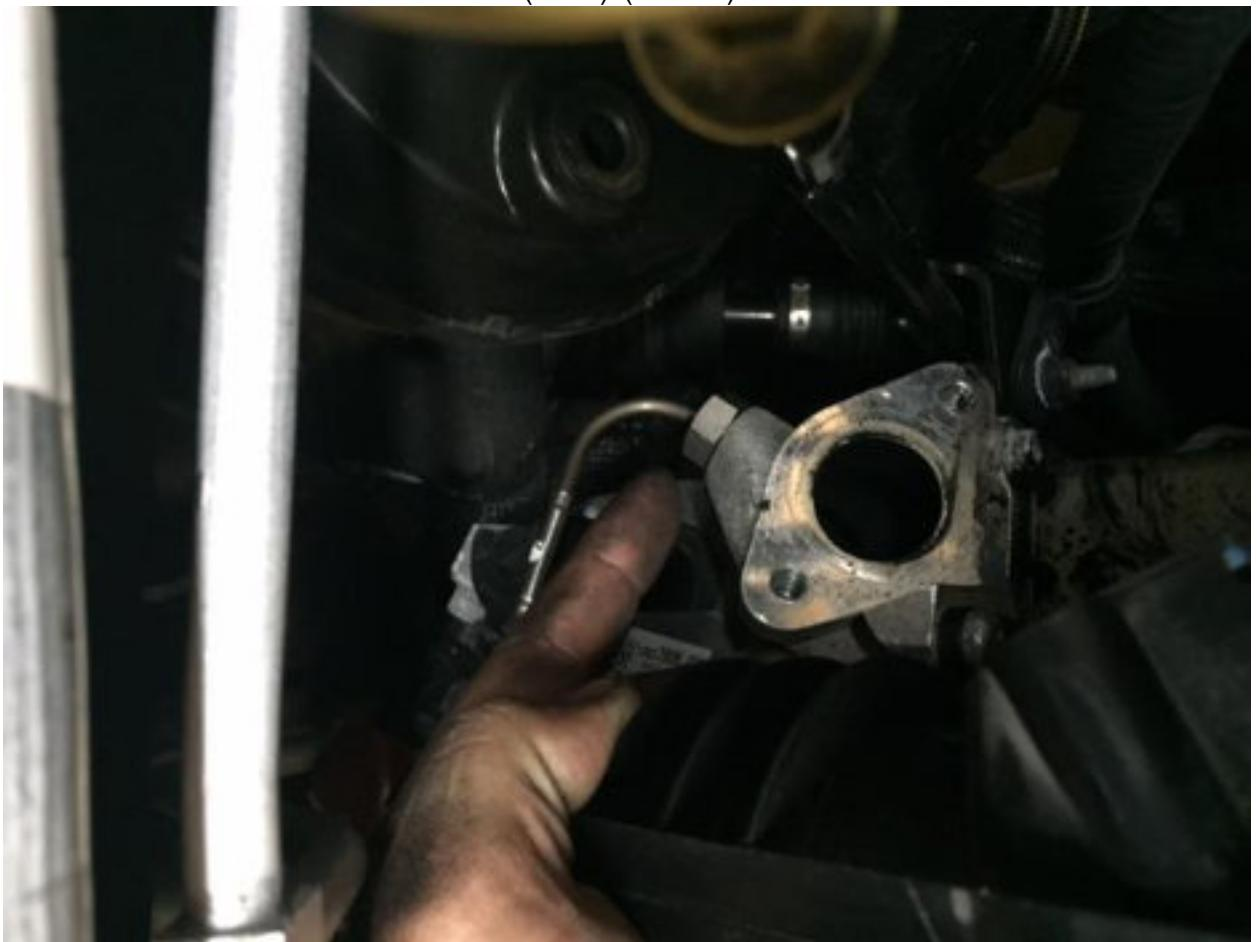
20. REMOVE WIRING HARNESS NUT (10MM)
