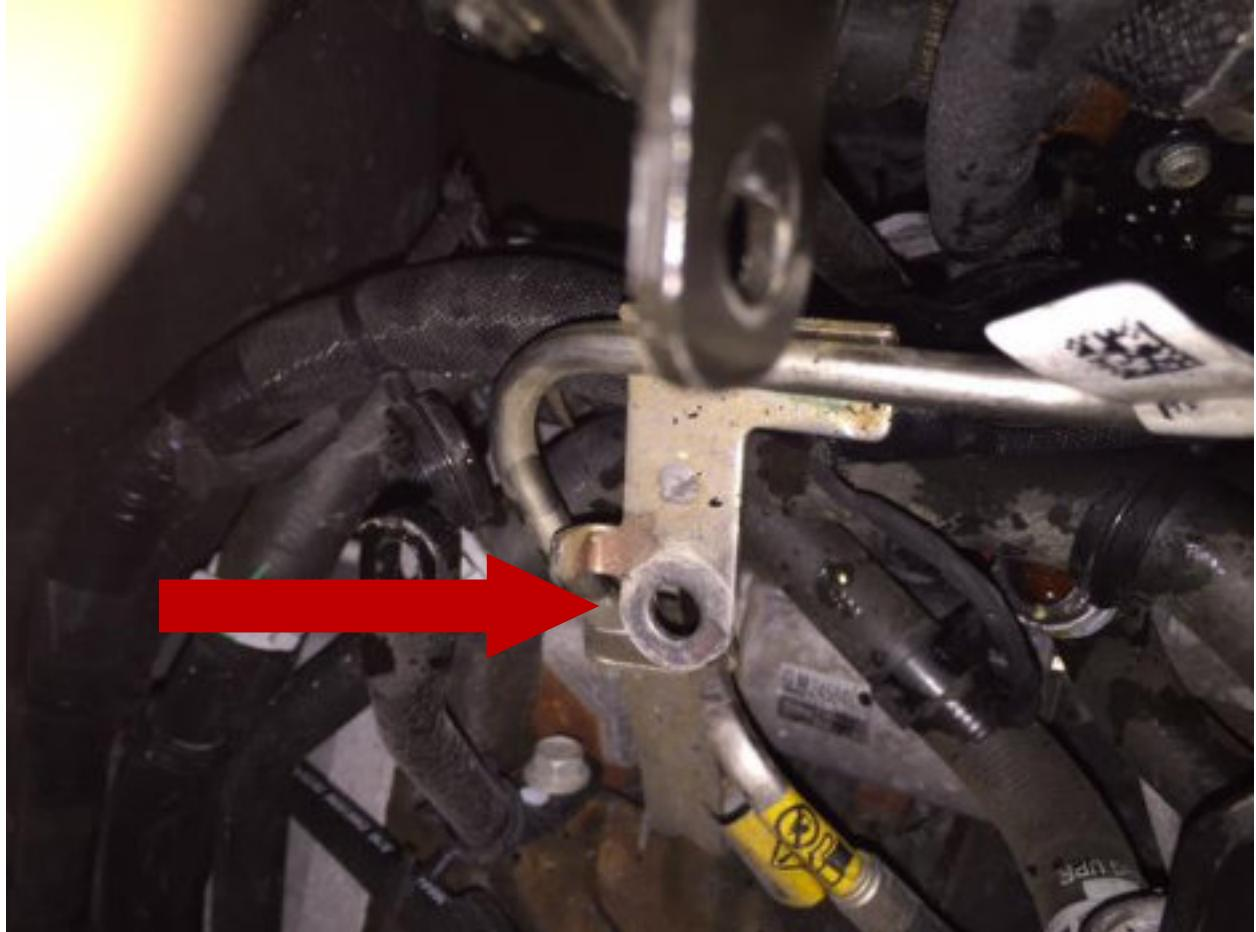
30. REMOVE EGR SUPPORT BRACKET BOLT (1 BOLT, 15MM) (ITEMS #21, 22)
