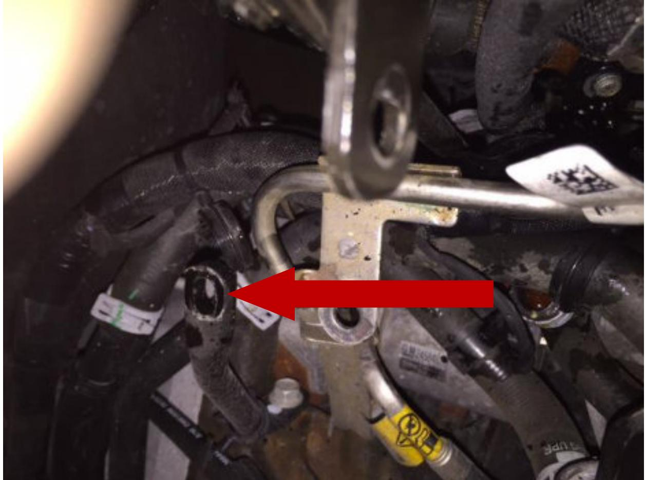
31. REMOVE DIP STICK TUBE (1 BOLT, 10MM)
