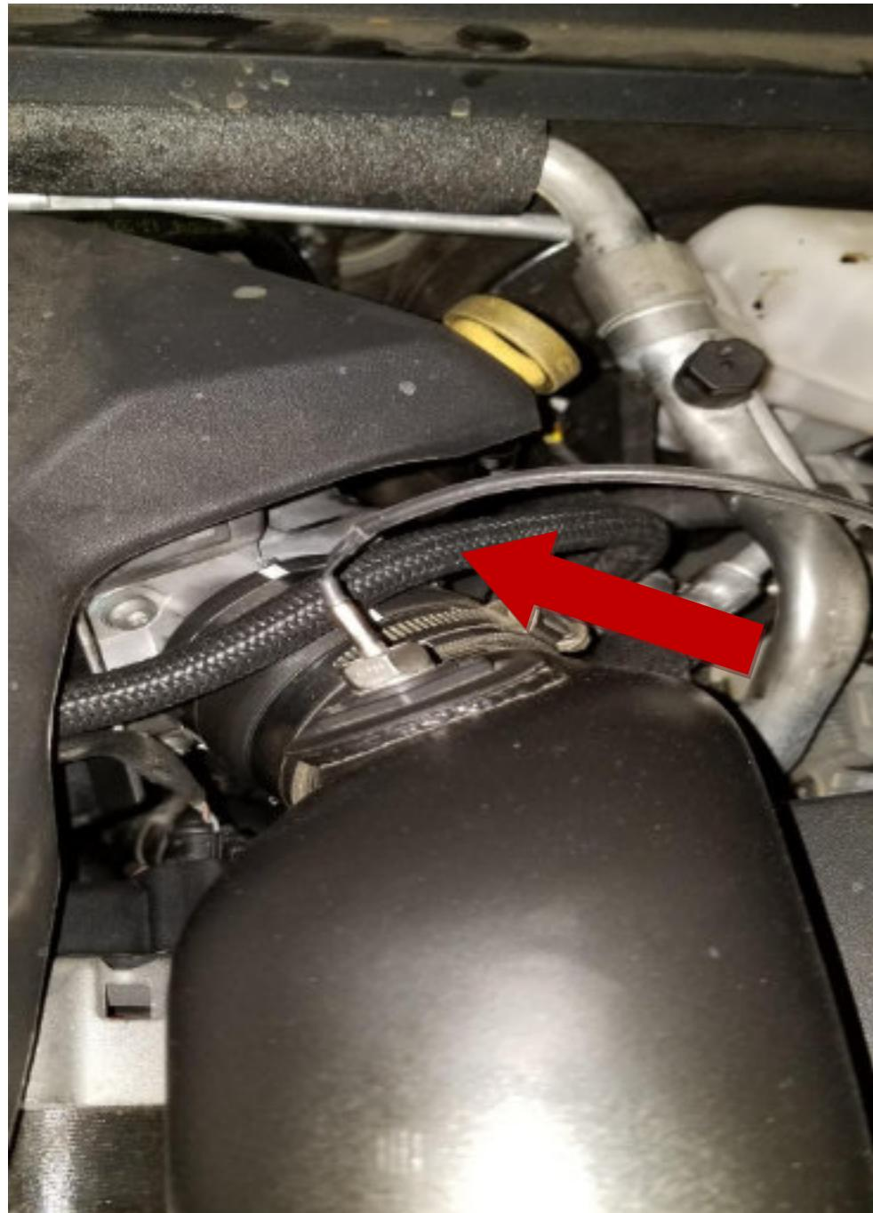
6. DISCONNECT FUEL FEEDLINE (3/8" FUEL LINE REMOVAL TOOL)
