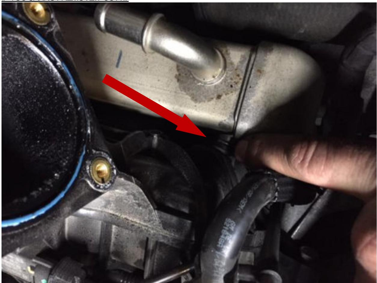
27. REMOVE LOWER COOLANT HOSE BARB FROM EGR HOUSING (1 BOLT, T30) (ITEMS #19, 20)
