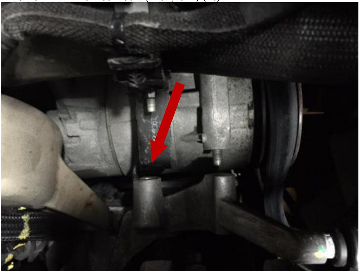
17. REMOVEFRONTEGRCOOLERMOUNT(1 BOLT, 13MM) (PIC) (ITEM 26)
