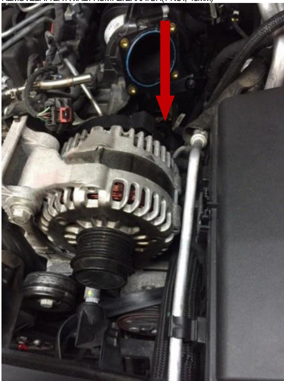
11. REMOVE BOLTS FROM ALTERNATOR (2 BOLTS, 15MM) (PIC)
