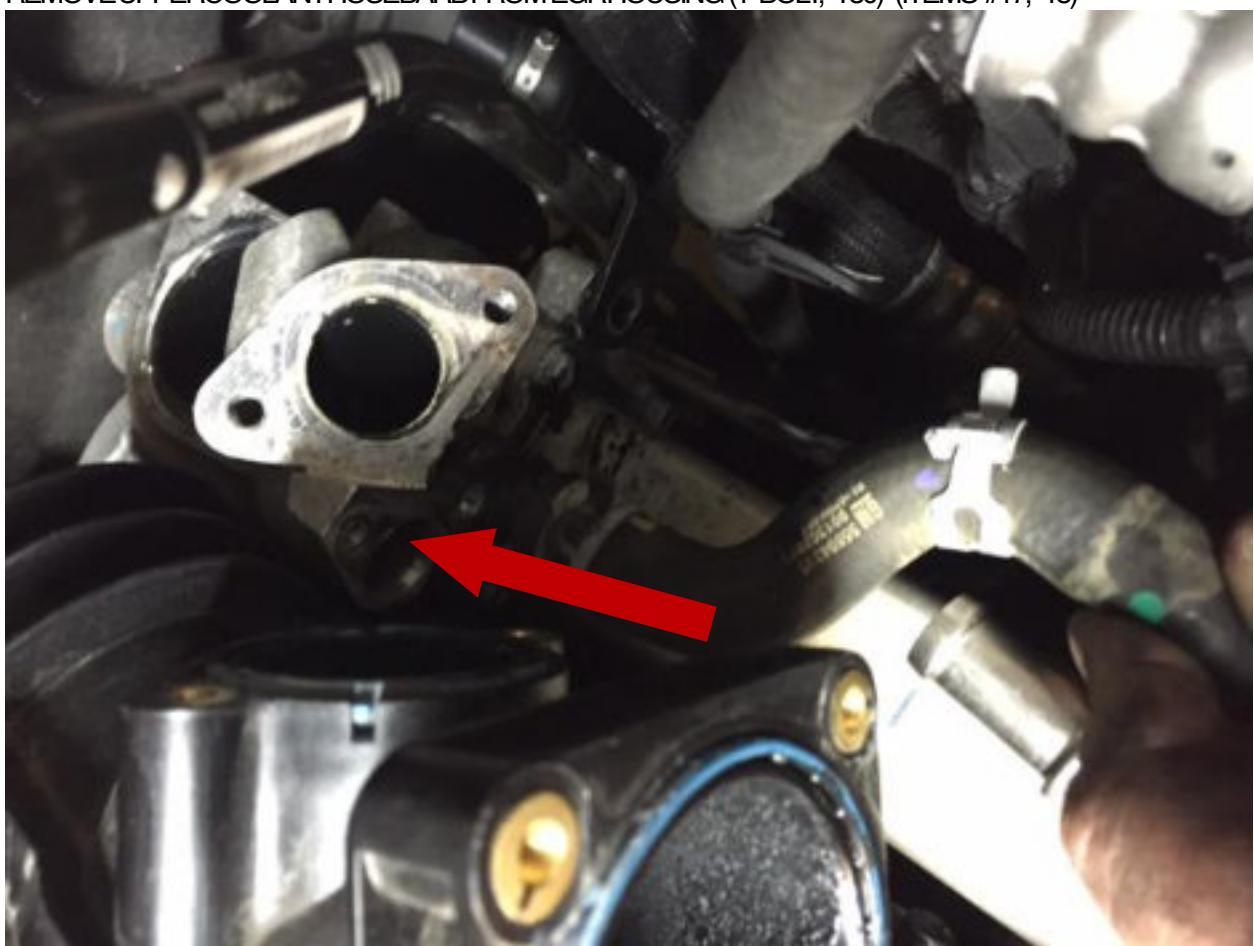
25. REMOVE EGR COOLER FROM EGR HOUSING (6 BOLTS, 5MM ALLEN) (PIC) (ITEMS #27, 28)
