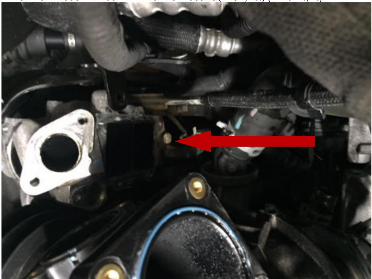
28. REMOVE EGR MIXING VALVE VACUUM LINE (CAPOENVALVE) (PIC) (ITEM #11)
