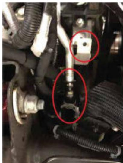
This hardline also has a smaller diameter line welded to it that feeds coolant to the urea Injector, these small rubber lines also need to be disconnected from the line so that it can be removed completely. Here is the assembly removed;
