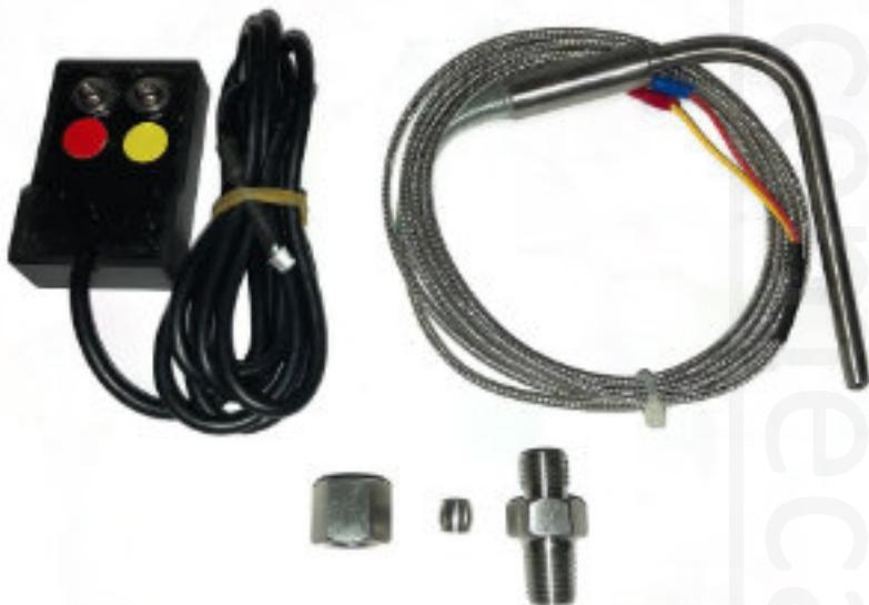
The RacemeUltra EGTProbe kit consists of three main pieces. The Module, the Probe, and the fitting. It is recommended the module be mounted inside the truck with the rest of the tuner components. This practice will prevent the small white four wire connector from being damaged while trying to push it through the firewall. The module plugs into the white four pin socket in the end of the controller. Before making this connection, it is recommended the OBD2 connector be unplugged from the port.
