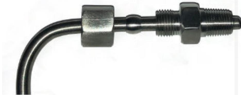
Once installed, slide the probe through the nut, then ferrule, then fitting and tighten the nut to secure the probe. Do not overtighten. In most cases, you can sink the probe until the 90 deg bend is at the fitting. This will ensure the sensing part of the probe is in the direct line of the exhaust flow.
