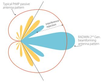
JET DUO beamforming antenna pattern vs. a typical PtMP antenna
