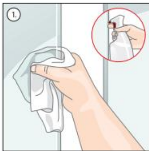
1. Clean glass edges with pure alcohol (Isopropanol/Ethanol), free of any additives.
