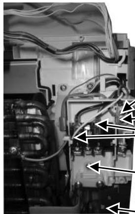
2. Release the 2 screws of the earth grounding terminal.
