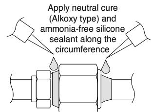
Neutral cure (Alkoxy type) & ammonia-free silicone sealant is only to be applied after pressure testing and cleaning up by following instructions of sealant, only to the outside of the connection. The aim is to prevent moisture from entering the connection joint and possible occurrence of freezing. Curing sealant will take some time. Make sure sealant will not peel off when wrapping the insulation.
