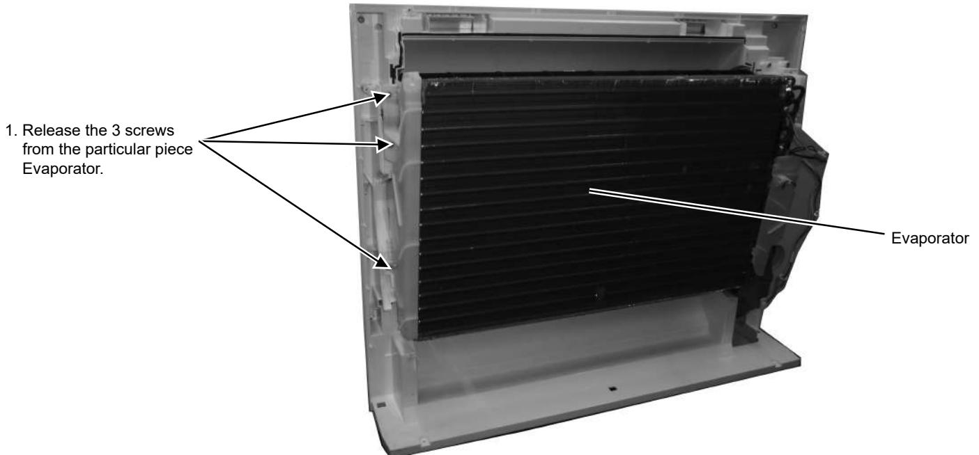
1. Release the 3 screws from the particular piece Evaporator.
