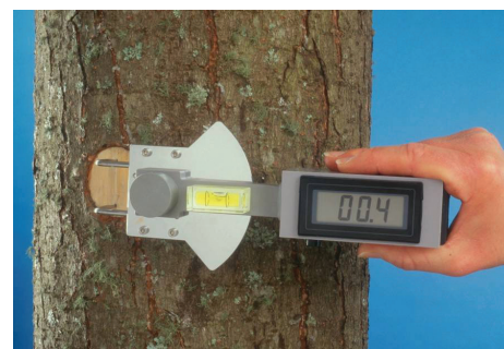
Fig 4: MoE being measured using an ST300.
