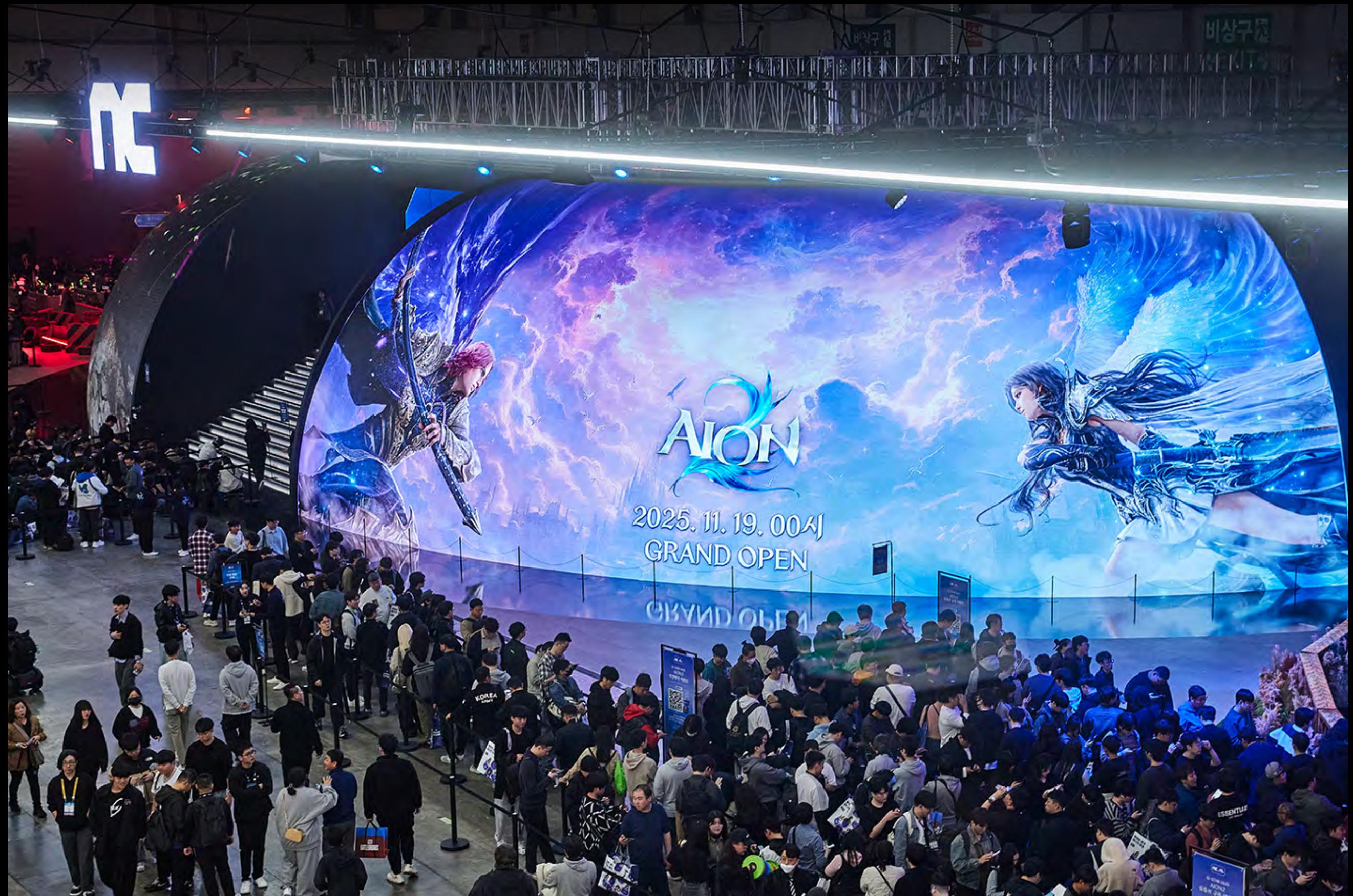
For the NCSOFT project, a total of 18,016 tangerine-peel modules were used for the dome alone. The structure measures 44 m in width and 8 m in height. On-site installation was completed over three days, with a rotating crew of approximately 100 personnel.
