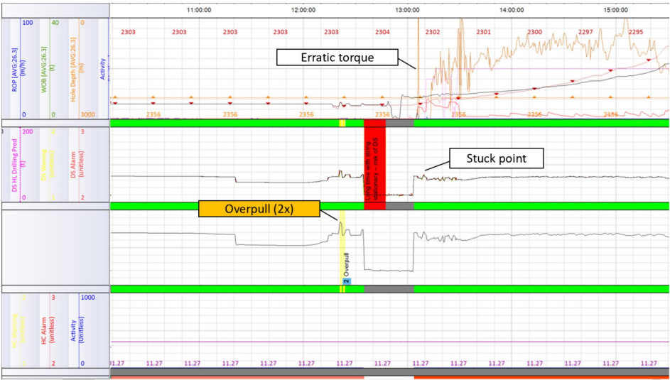
Figure 9—Case 6: Mechanical Sticking risk detection module provided warnings due to observed overpulls before the stuck pipe on May 30 th .
