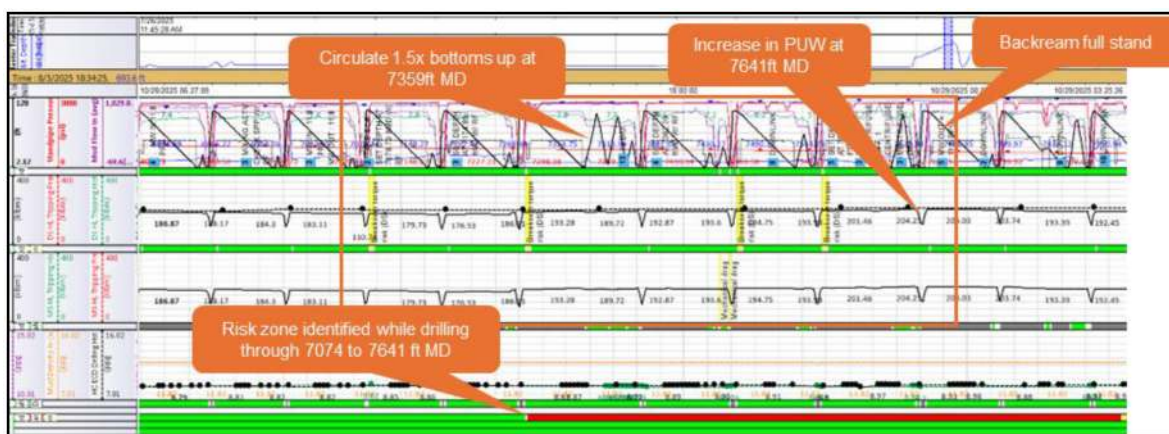
Figure 11—Agent output during drilling from 7,074 to 7,641 ft MD, with multiple BOT and mechanical drag warnings identifying the DS risk zone and the corresponding increase in Pick-up Weight (PUW) at 7,641 ft MD.
