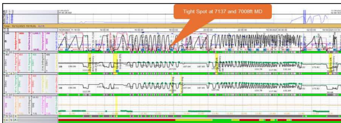
Figure 12—Tight spots encountered at 7,137 ft MD and 7,008 ft MD during pumping out of hole, within the same risk interval identified during drilling (fig.10).
