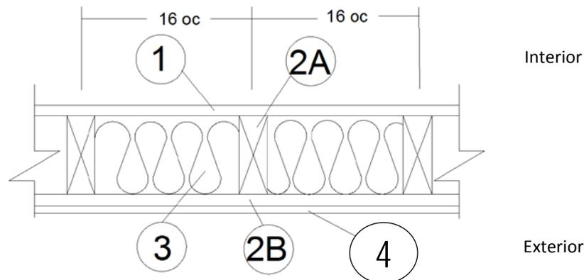
**1. GYPSUM BOARD (Interior):** One layer Type X, complying with ASTM C1396, min. 5/8 in. thick, 4 ft. wide applied vertically, fastened to framing. Joints covered with paper tape and joint compound. Fasteners covered with joint compound. Min. #6 × 1-5/8 in. long Type S or W screws, spaced max. 6 in. on center (oc).
