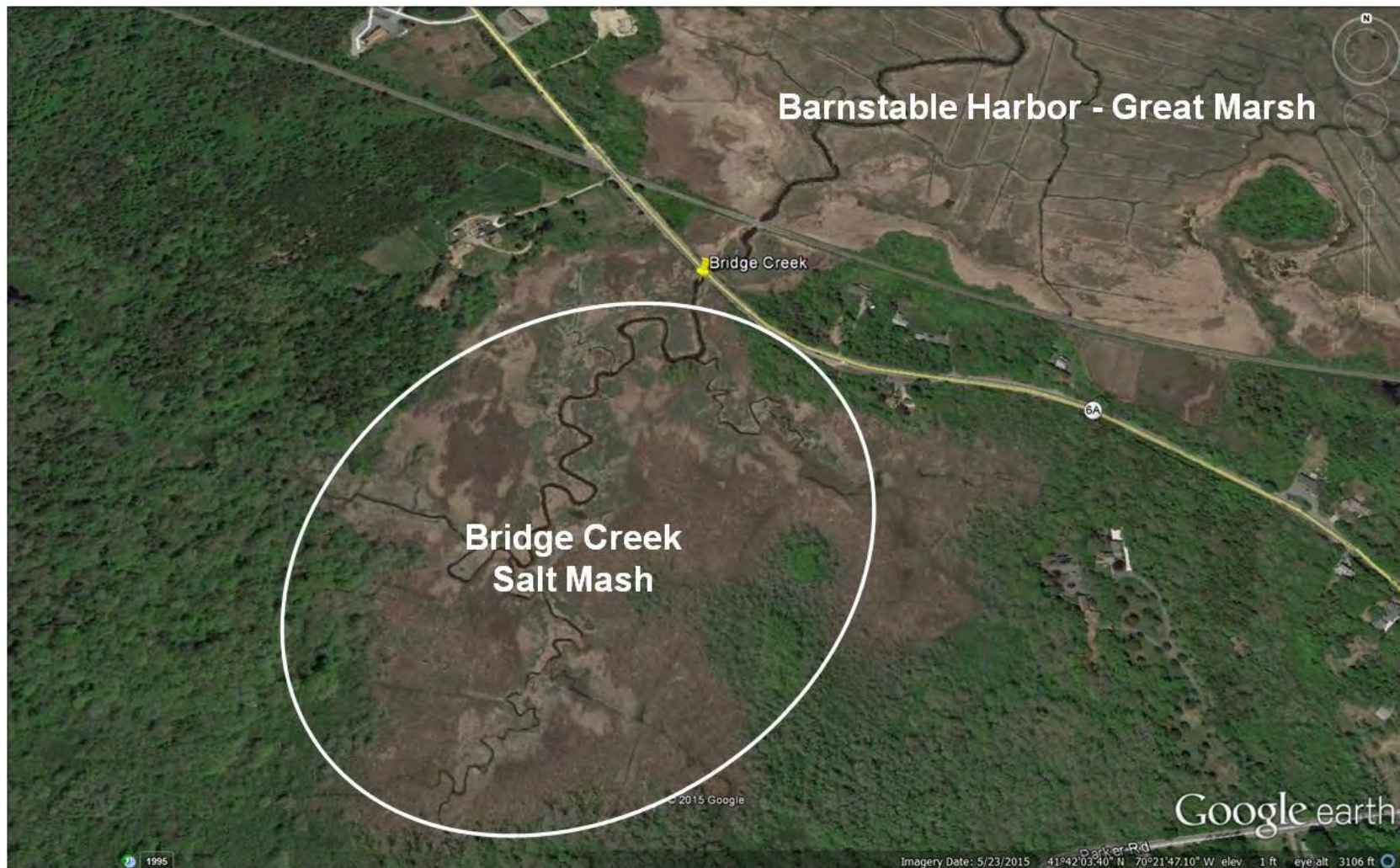
Figure IV-11. Location of MEP stream gauge (yellow symbol) for measuring flow and nitrogen load in Bridge Creek. The Bridge Creek salt marsh receives groundwater flow from surrounding wooded upland and discharges to the down gradient estuarine receiving waters of Barnstable Harbor-Great Marsh.
