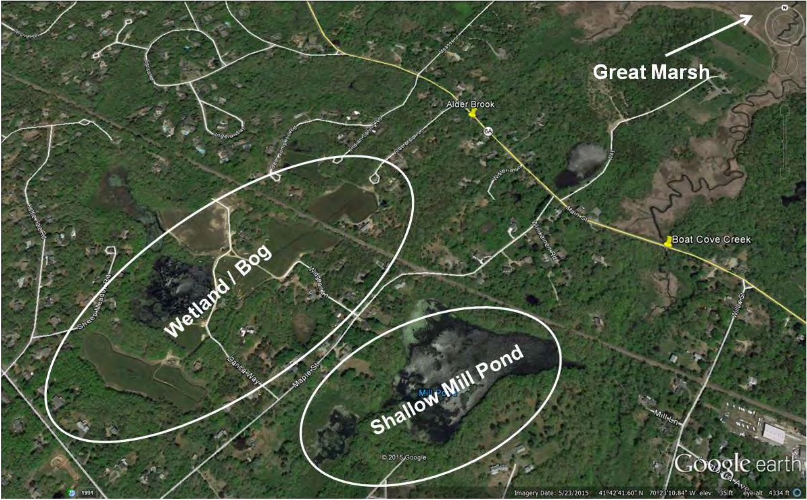
Figure IV-8. Location of MEP stream gauges (yellow symbol) for measuring flow and nitrogen loads transported by Alder Brook and Boat Cove Creek to estuarine waters. Alder Brook receives surfacewater from a upgradient bog/wetland feature whereas Boat Cove Creek discharges from a shallow up-gradient pond.
