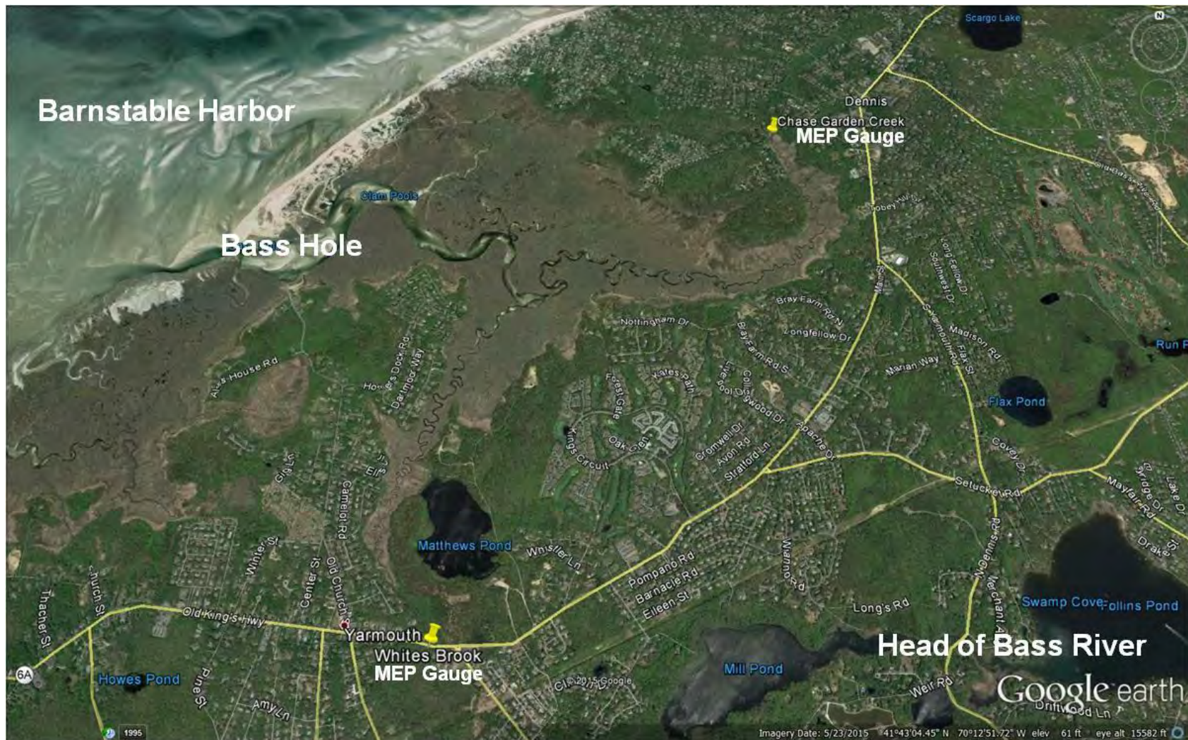
Figure IV-15a. Location of two MEP stream gauges (yellow symbol) on streams discharging to the Bass Hole sub-embayment (southern stream is Whites Brook and northern stream is Chase Garden Creek). Freshwater flow and nitrogen load were measured over a complete year at each gauge site. Bass Hole is a major tributary to the Barnstable Great Marsh estuary system.
