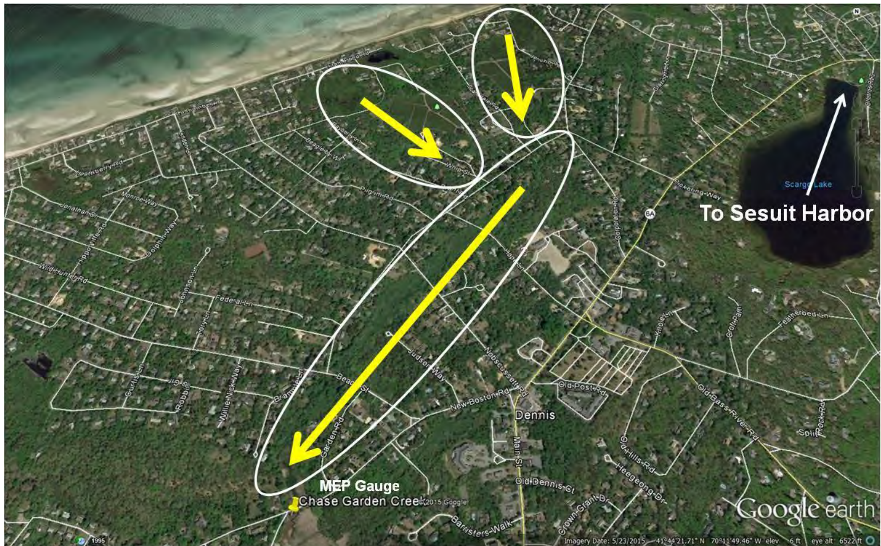
Figure IV-17. Location of MEP stream gauge (yellow symbol) for measuring flow and nitrogen load in Whites Brook. Yellow arrows show the direction of surfacewater flow draining a marshy riparian zone along Chase Garden Creek as well as a network of bogs as the head waters of the Creek.
