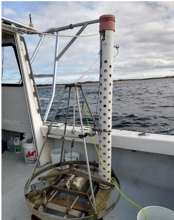
Figure 2. Young-Modified Van Veen Grab Sampler onboard the R/V Marindin
