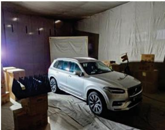
Test setup in RC with car*.
