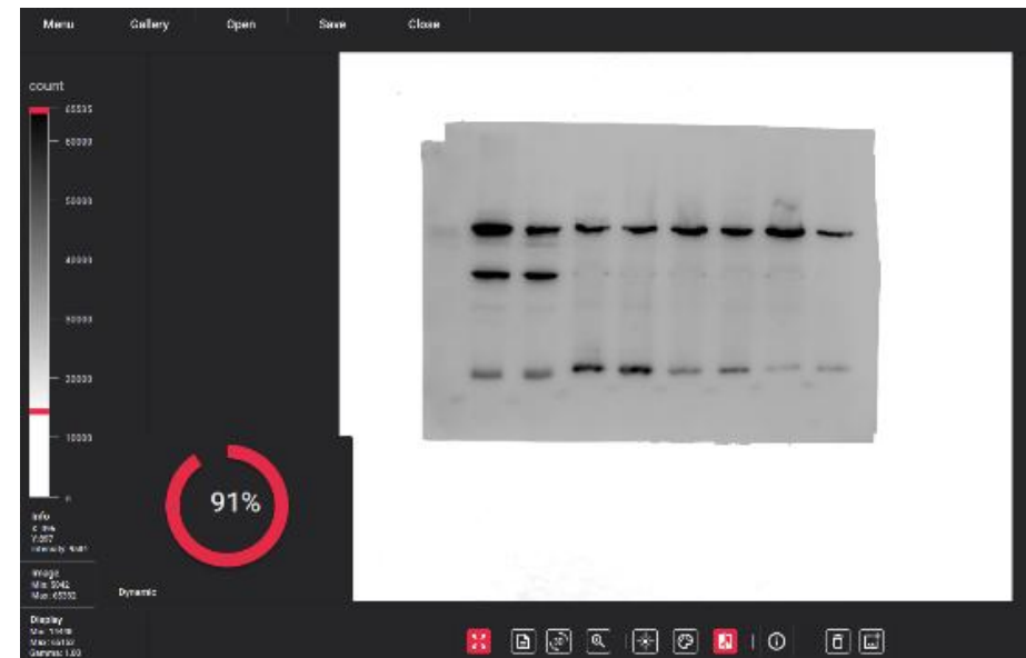
Figure 4: Percentage representation of greyscale levels. Out of 65,536 grey values, 91% are represented ensuring user that quantification is precise and reliable.
