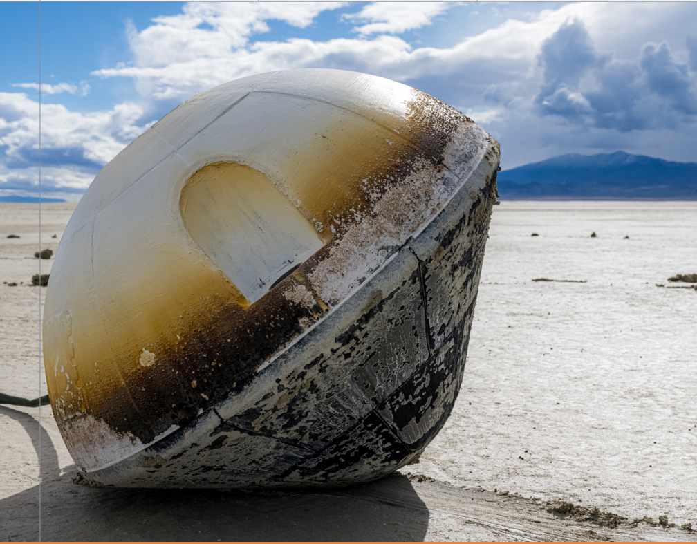
Varda's W-1 capsule after successful orbital reentry and recovery in Feb 2024
