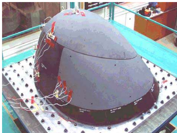
Figure 26 C-SiC Nose (courtesy IRS).
