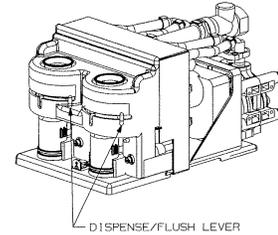
**IMPORTANT:** When making changes to the water flow control, do not rotate more than 1/4 turn per adjustment. Additionally, prior to taking your next brix reading, “tap” the corresponding dispense button several times prior to drawing a sample. This will clear remnant drink from the dispense nozzle AND help move the flow control to its new setting.
