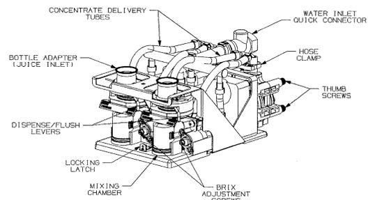
3. Flush the system prior to removing the pump platform (refer to the Daily section located at the beginning of the Planned Maintenance Schedule). Remove the dispense nozzles and static mixers.
