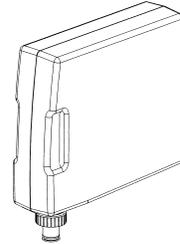
**NOTE:** Be sure to lubricate the o-ring seal on the container nozzle. This will ensure a good seal and allow the pumps to draw concentrated from the containers more easily. Failure to create a good seal at this connection may result in weak drinks and/or seepage of concentrate.
