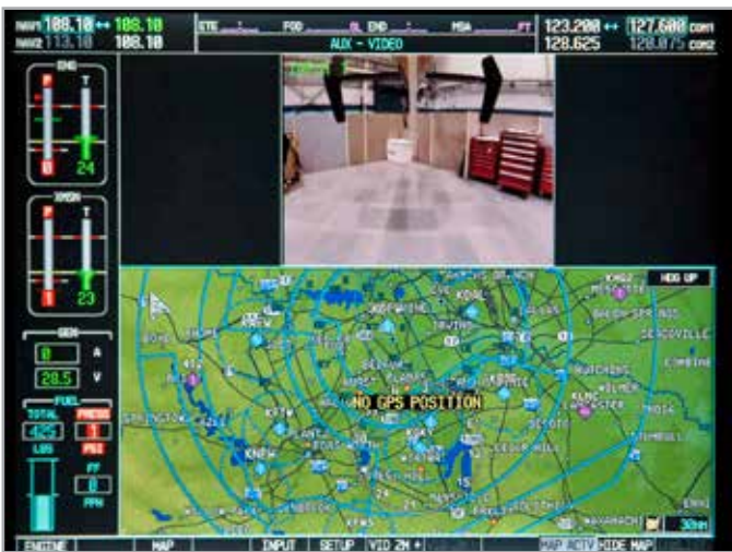
MFD Tail Rotor Camera / Map Display.
