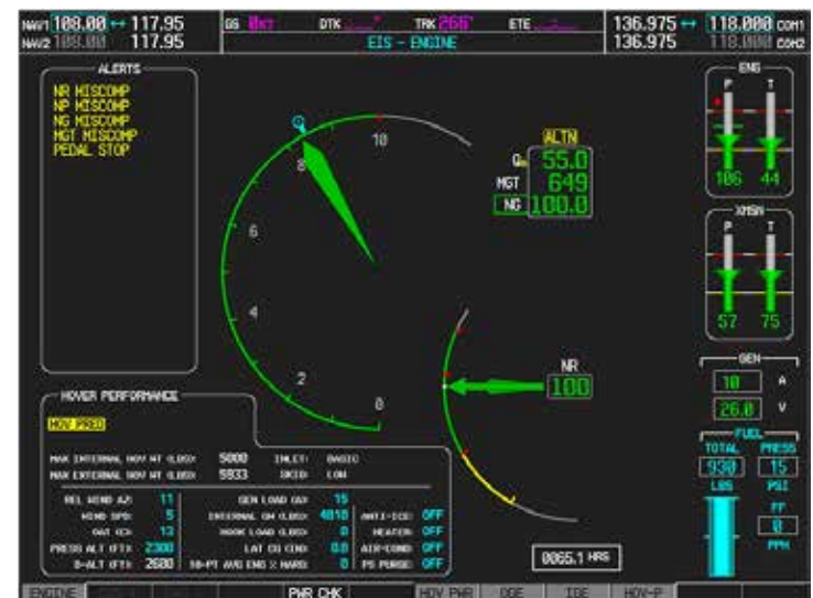
Pre-flight planning hover performance check (HOV-Predictive Mode).
