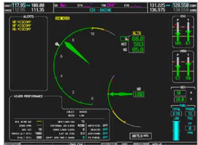
MFD Power Assurance with HOGE performance in real time mode.
