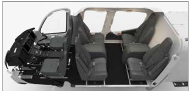
Four place club seating with two 21.5" seats separated by a center console in each row.
