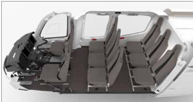
Standard six place 15.5" wide passenger seats in forward facing airline seating arrangement.
