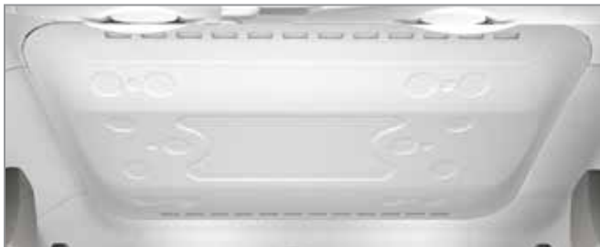
Standard headliner with slotted air vents.
