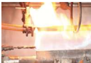
RESISTANCE TO FIRE ALONE TEST (CATEGORY C)
