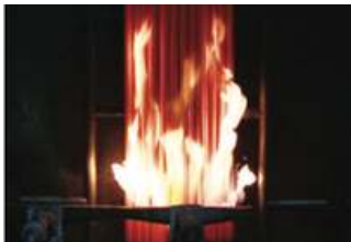
FLAME PROPOGATION TEST (IEC 60332-2)
