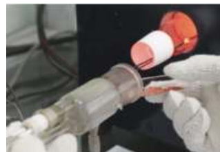
ACIDITY & CONDUCTIVITY TEST (IEC 60754-2)
