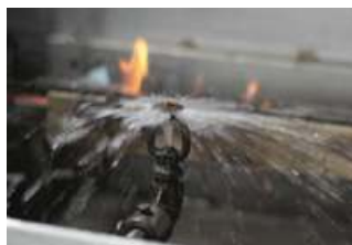
RESISTANCE TO FIRE WITH WATER TEST (CATEGORY W)
