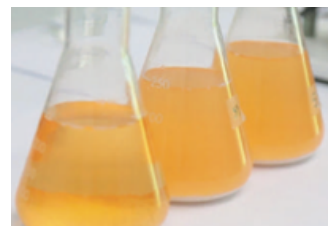
HALOGEN ACID GAS CONTENT TEST (IEC 60754-1)
