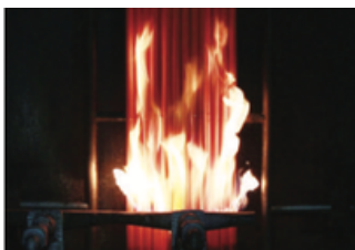
FLAME PROPAGATION TEST (IEC 60332-2)
