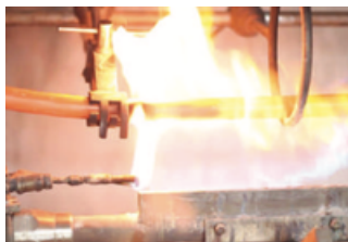
RESISTANCE TO FIRE ALONE TEST (CATEGORY C)
