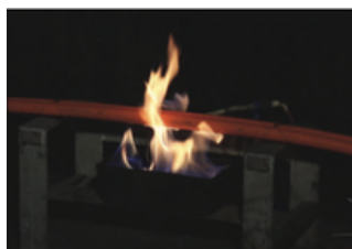
SMOKE DENSITY TEST (IEC 61034)
