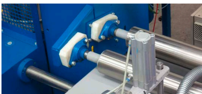
Sensor type RR W to measure over the full fabric width on two rollers
