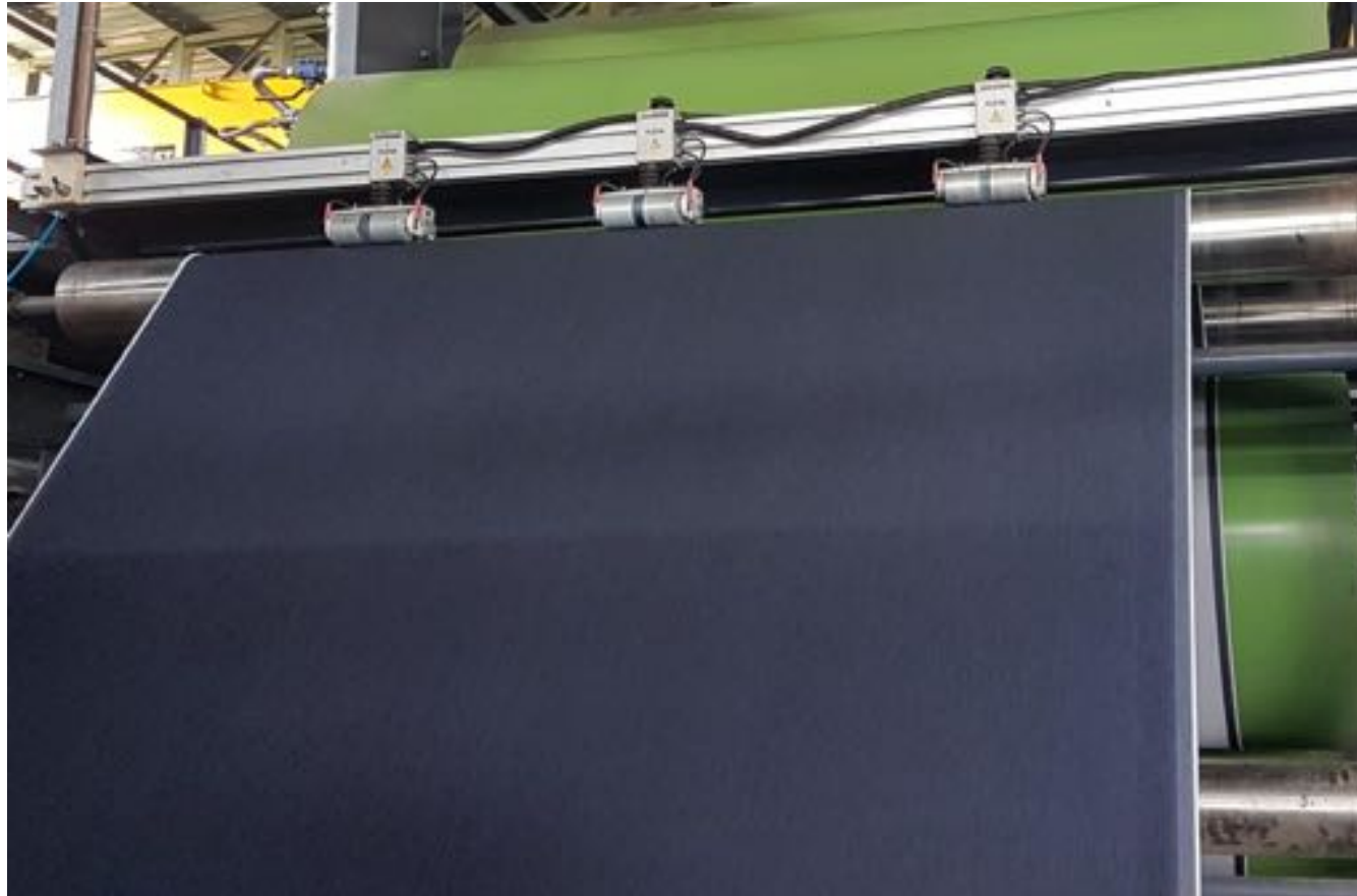
RR 3.3 after cylinder dryer before sanforizing
