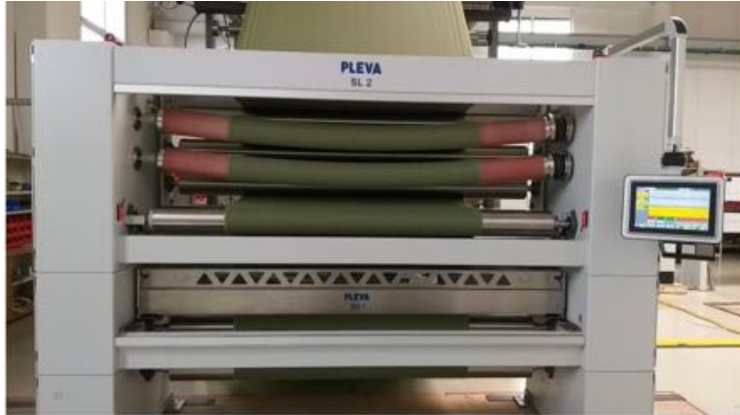
Straight Liner SL 2 – reinforced version for denim
