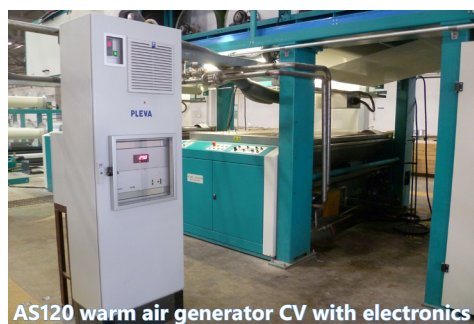
AS120 warm air generator CV with electronics
