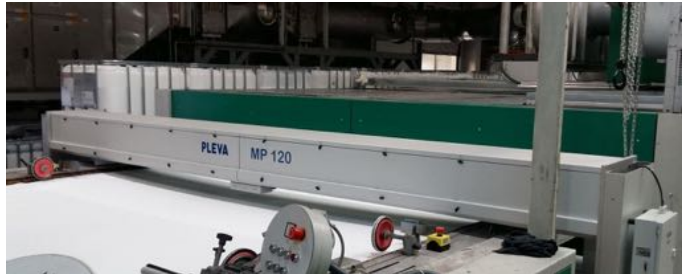
Traversing measurement MP120 after knife coating
