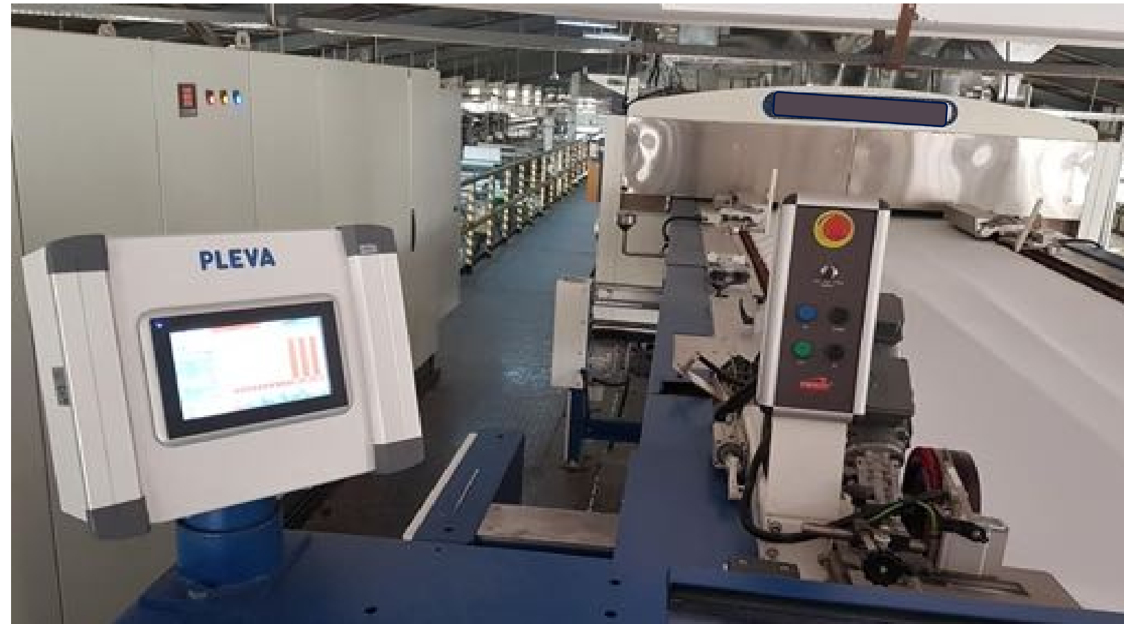
PLEVATEC smart 7 / smart 10 installation at stenter frame
