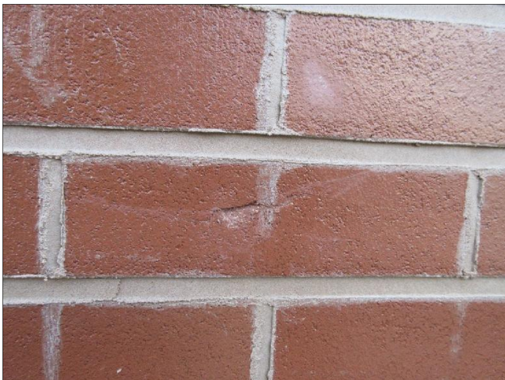
10 Nm HARD BODY IMPACT - SMALL CHIP FROM BRICK FACE
