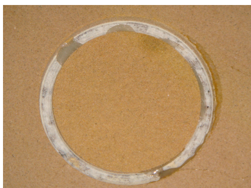
Pull-off tested Aerolite cladding panel specimen post weatherometer testing. Failure occurred within the sandstone facing material.
