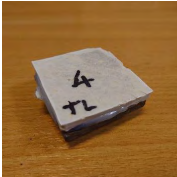
Plate 8 - Typical Sample where Failure Mode is Between the Veneer and Honeycomb Layers
