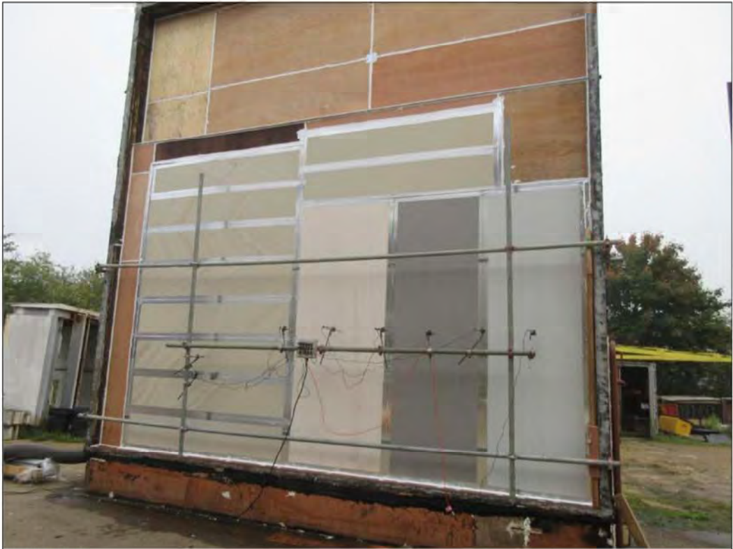
TEST SAMPLE DURING WIND LOADING
