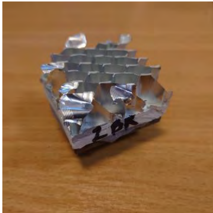
Plate 7 - Typical Sample where Failure Mode is in the Honeycomb Layer
