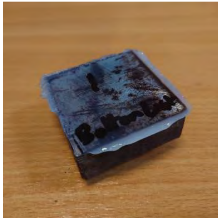
Plate 9 - Typical Sample where Failure Mode is Between the Plate and Veneer Layer
