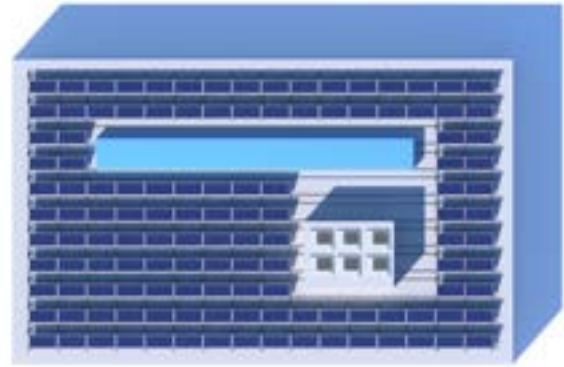
The centre section of the roof is the best place for the solar panels. No panels should be fitted in areas where shadows are cast.
